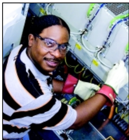
Maurice Taylor services the power board for an 8-axis mill.
