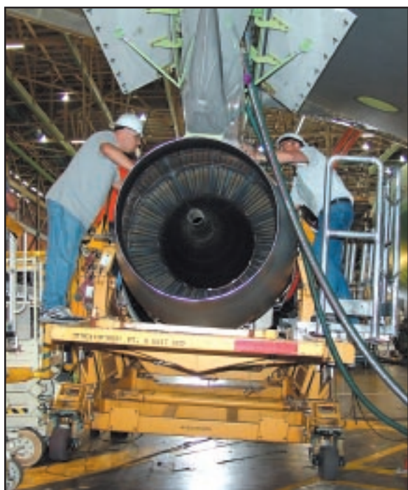
Tooling members designed and built a platform (right side) so members no longer work on a 4-inch beam (left side) while hanging engines.
