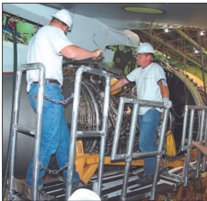
Photo above: On the new platform, members can not only walk around, but safely put the required torque on the bolts to secure the engine.
