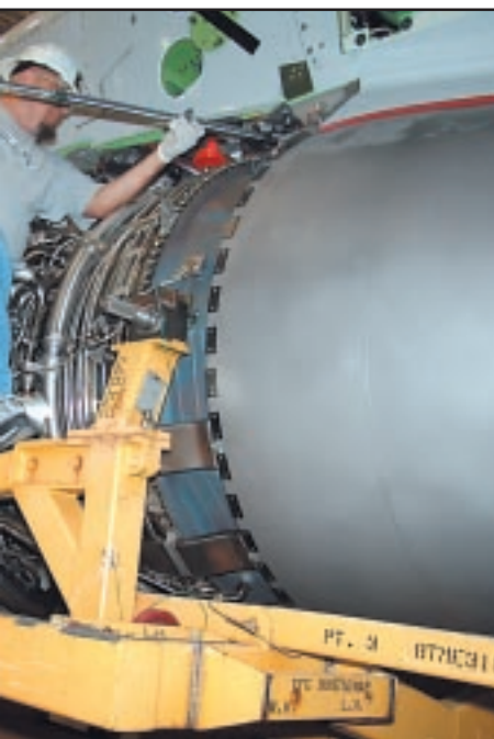
...employees hanging an engine worked on a ...p while putting 350 pounds of torque on ...the ankle is twisted for balance.
