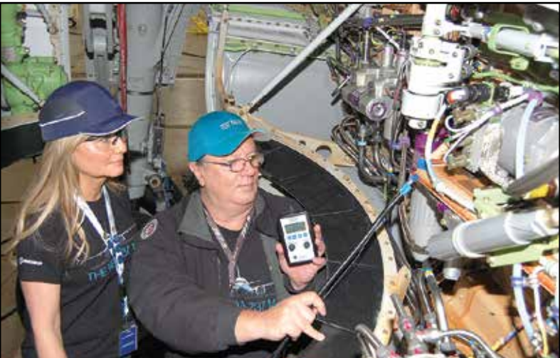
Union Steward Chris Black (r) and materials engineer Kathy Ferguson are part of a FOD Buster team that invented a way to locate lost tools in minutes rather than days using an electromagnetic field detector to find a previously magnetized tool.
