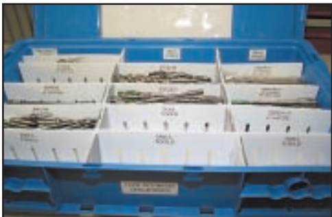
Kits from Auburn CTSC contain all tools needed for a job, as well as slots to return dull parts to be resharpened.
