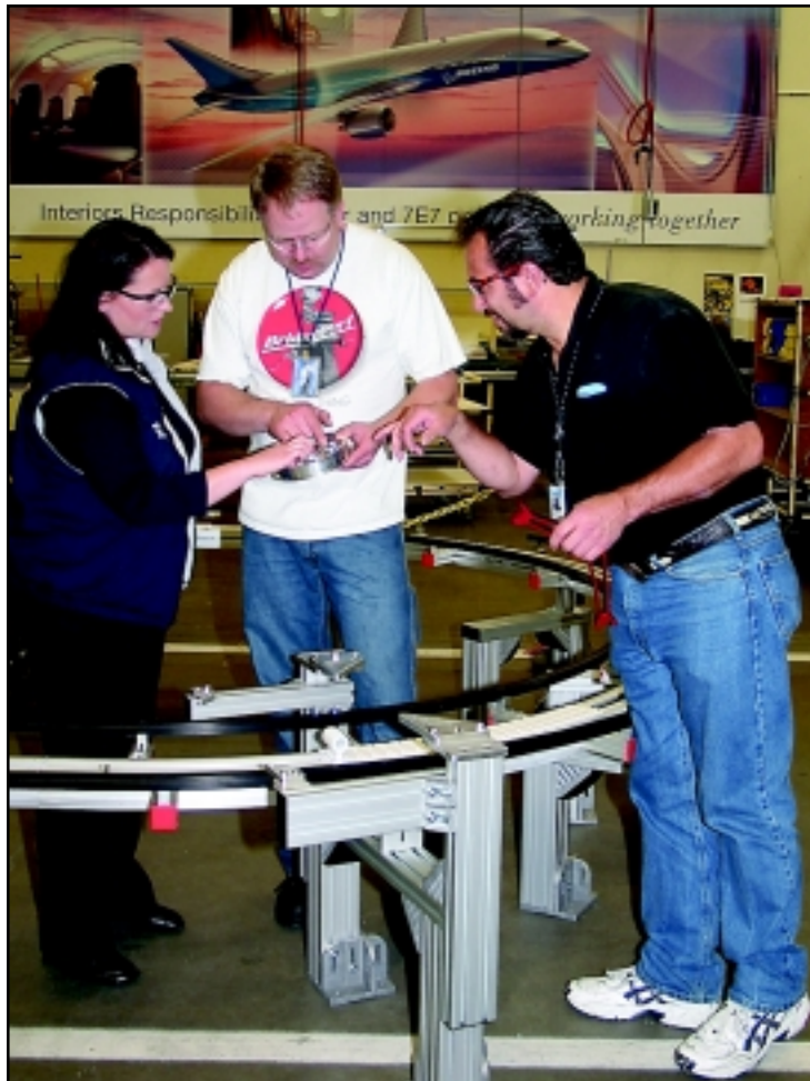
K.C. White (center) and Geno DeBartole show Business Rep Heather Barstow some of the custom machine work IRC did on the new moving line. Geno played a vital role in designing and building the moving line while K.C. did much of the custom machine work.
