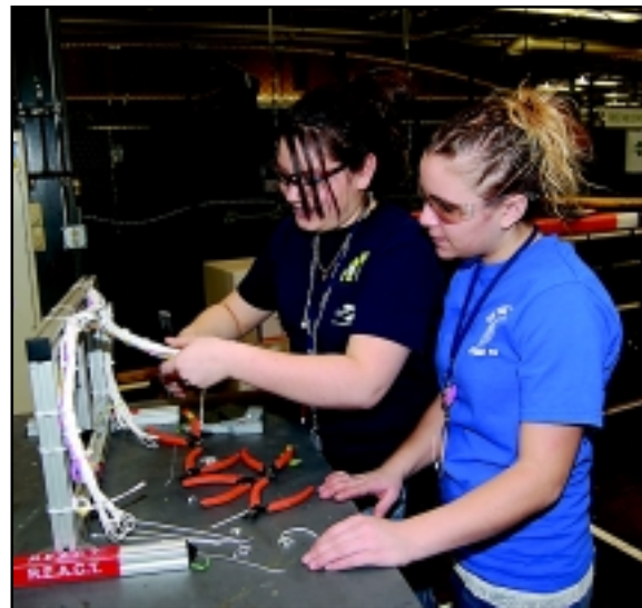
Tiffany Oschip (l) and Ashleigh Donner try different cutters designed to avoid damaging wires when it is necessary to cut into the bundles on the plane.
