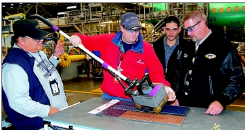
L to R: Phil Larvie, Steven Long, and Marc Honda (manager) show Business Rep Tommy Wilson the roller they designed to install galley mats in the 737. This solved a bubbling issue that engineers had been unable to resolve. These members are part of a brainstorming group established to help with similar issues using the skills and knowledge of our members.
