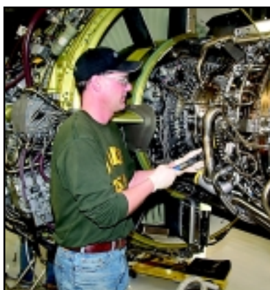
Jay Stendahl prepares a 737 engine to hang on the plane.
