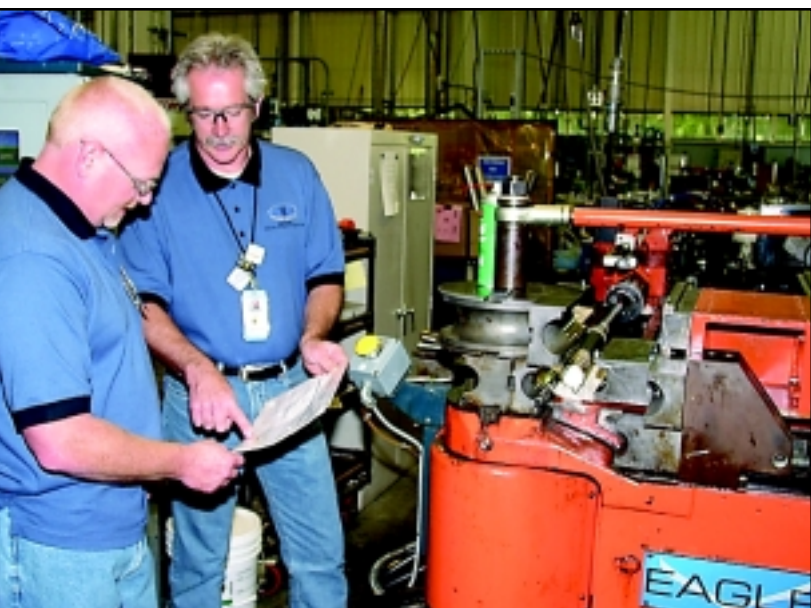
Site Safety Committee members Clark Fromong (l) and Brett Coty revised Operating Procedures to make the tube benders safer. In addition, machine guards and a pressure sensitive mat will be added.
