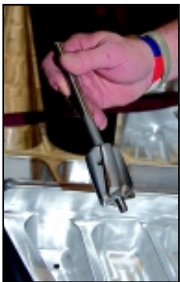
Doug Wilke designed this spot face cutter to use on the pickle forks.
