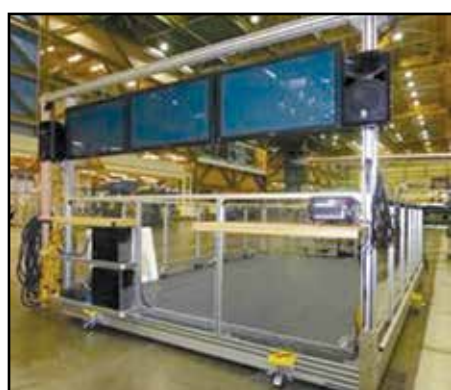
Electrical issues stemmed from these barges or portable offices built to hold 10 computer stations, printers, copiers and flat screen displays with no regard on how to power the barge.
