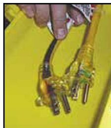
Our electricians discovered one cord had already burned the neutral prong and could easily have caused a fire.
